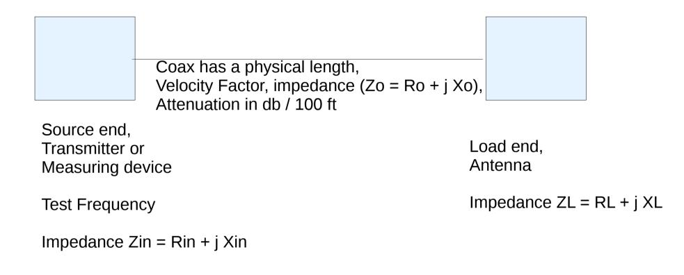
Typical use is to compute Load Impedance after measuring Zin.
