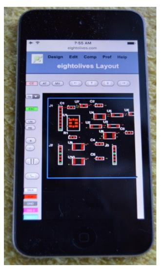
A web tool for circuit board layout.
